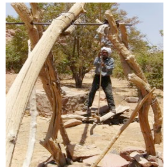
Old fashioned ‘shadoof’ requires the water tank to be beside the well. Many gardens must use a oil pump to reach a water tank at a higher level in their gardens.
